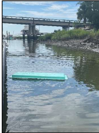
Figure 11: Simulation of fish box lid floating in Savannah River, GA, to show little to no sail area. Source: USCG.
