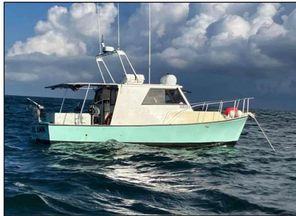
Figure 13: F/V CAROL ANN life raft stowed underneath a-frame radar mount Source: F/V CAROL ANN owner's Facebook.
