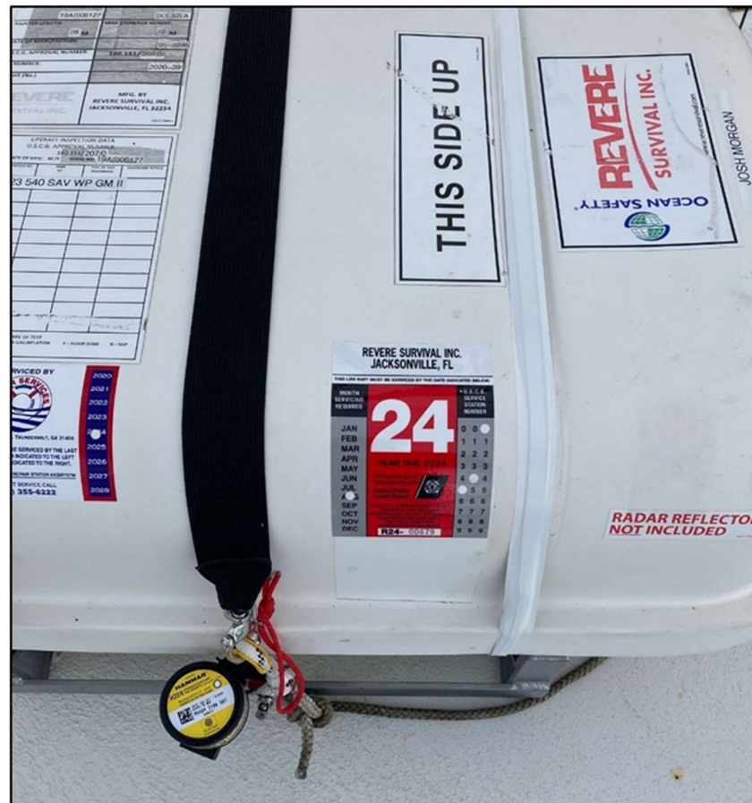
Figure 6: Properly rigged Coast Guard approved life raft on the F/V CAROL ANN. Source: USCG.
